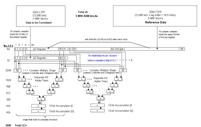
The <u>single</u> Multiply-Add-Accumulate structure in the lower left of the diagram above produces, in one clock, a single <u>partial</u> (16 complex multiples, summed) output sample.
